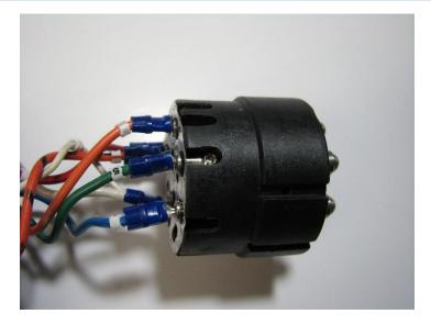
Per the picture above, loosen (but do not completely remove) the small set screws holding the wires into the spring loaded pins.
