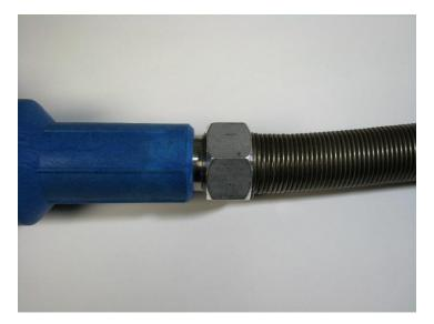
Per the picture above, loosen the large nut on the strain relief.
