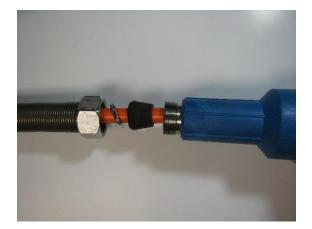
Per the picture above, slide the new rack cord through the strain relief spring and nut, then through the metal backup ring and rubber grommet and through the rack plug body.
