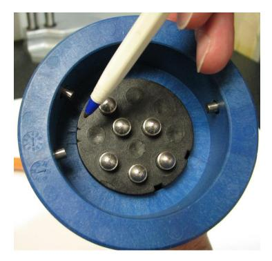
Rotate the contact block as needed to take up excess wire and insert the contact block into the rack plug body such that the (2) index marks on the black plastic contact block align with the (2) index marks on the rack plug body (see picture above).
