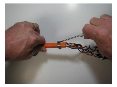
You can now remove the contact block from the cord. To remove the cord from the plug body you can loosen the clamp (see picture above) by inserting a screw driver in the crimped ears and twisting, or you can cut the cord off below the clamp so the cord can be removed through the strain relief.
